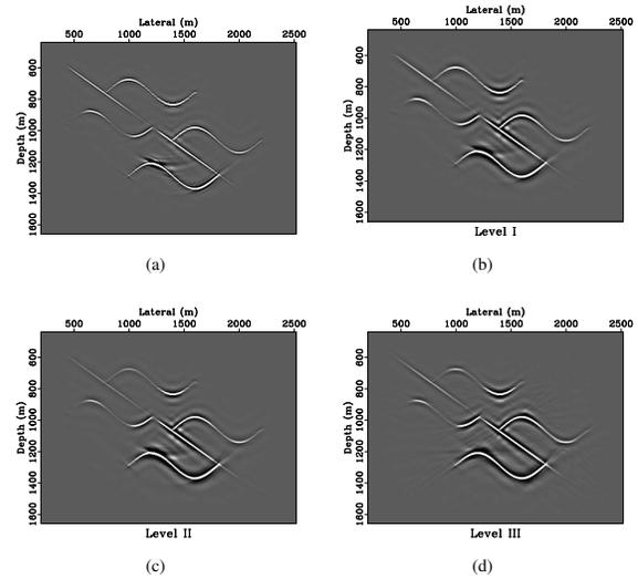
Figure 2: Different levels of preconditioning. (a) Migrated image without preconditioning—i.e.,  $\tilde{\mathbf{x}} = \mathbf{A}^* \mathbf{b}$ . (b) Migrated result for left preconditioning (cf. Equation 5). (c) Migrated result for left-right (depth-correction only) preconditioning (cf. Equation 6). (d) The same but now including curvelet-domain scaling (cf. Equation 9).
