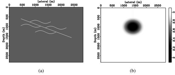
Figure 1: Synthetic example. (a) Reflectivity. (b) Low-velocity lens model used as a background velocity for both migration and modeling operators.
