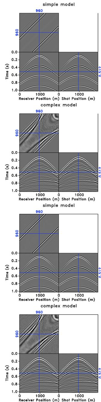
Figure 2: Comparison between conventional and compressive simulations in for simple and complex velocity models. **(a)** Crossing-planes view of the seismic line for the simple model. **(b)** The same for the complex model. **(c)** Recovered simulation (with a SNR of 28.1 dB) for the simple model from 25% of the samples with the  $\ell_1$ -solver running to convergence. **(d)** The same but for the complex model now with a SNR of 18.2 dB..
